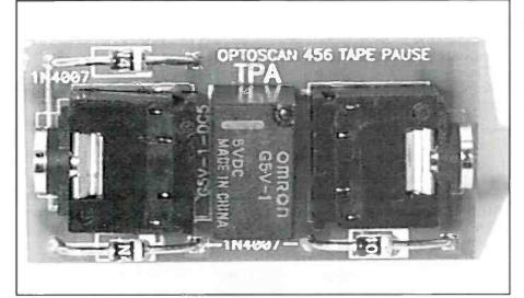
The OS-456 Tape Pause Adapter. You will need this if you're using an OS-456 interface and controlling a tape recorder with the software. If using a VOX recorder, there is no connection to the OS-456 tape remote jack.
