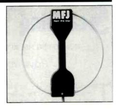
also available. The MFJ-1788 is also portable and can be mounted both vertically and horizontally. A heavy duty 1/8 inch thick ABS plastic housing with ultraviolet inhibitors protect the tuning unit from the weather. The MFJ-1788 does not need a ground, radials, counterpoise or antenna tuner. It will cover 40 through 15 meters continuously with low SWR and handle 150 watts.
