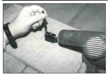
My son Tom shows how he is testing the capacitor for release with the drift punch while applying heat from a hairdryer. This is easy to do while the capacitor is installed on the chassis.
