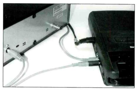
The BC-9000 XLT is one of few radios with an auxiliary control port for the recorder. The AUX from the radio is connected (with appropriate cables and adapters from RadioShack) to the REM jack of the recorder. Note that the LINE OUT jack on the Bearcat series is on the front panel.
